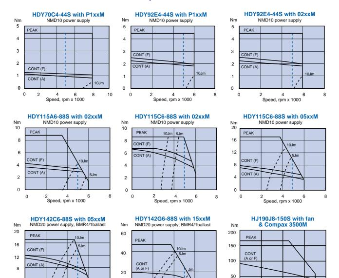
Note: Speed is limited to 5000rpm when using SV-M series drives (shown by broken blue line)
