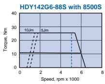
Note: Speed is limited to 5000rpm when using SV-S series drives (shown by broken blue line)
