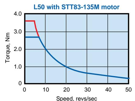
— Red lines indicate torque with boost applied
