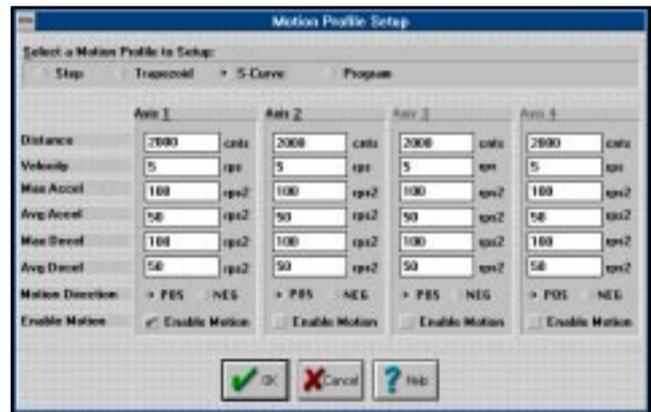
Pushing START will automatically cause the motion to initiate and the system response to be graphed in front of you. Capture and display up to nine motion parameters. You can even graph velocity vs. position.
