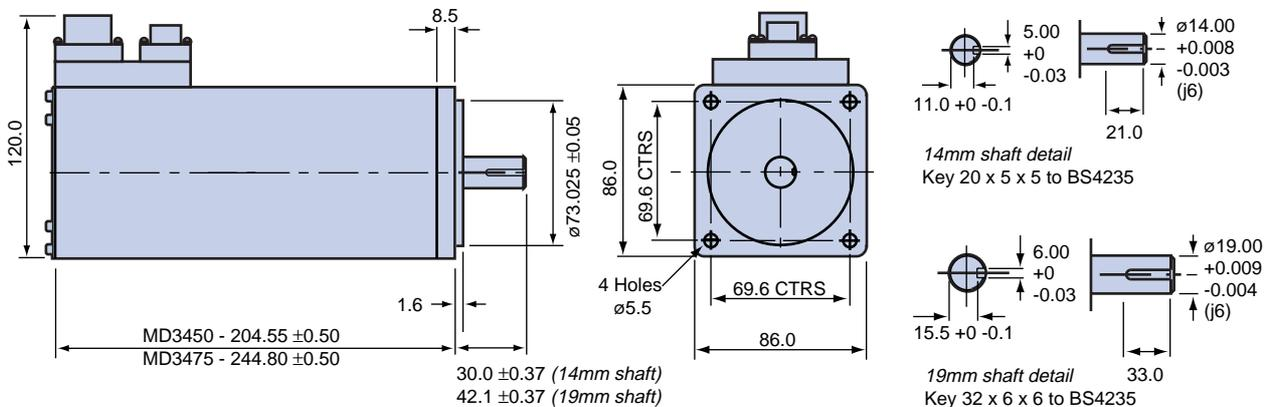
The 14mm shaft option is suitable for in-line coupling (e.g. leadscrew or gearbox) and for toothed belts up to 15mm wide. For toothed belt transmissions utilising the full motor power, the 19mm shaft is recommended.
