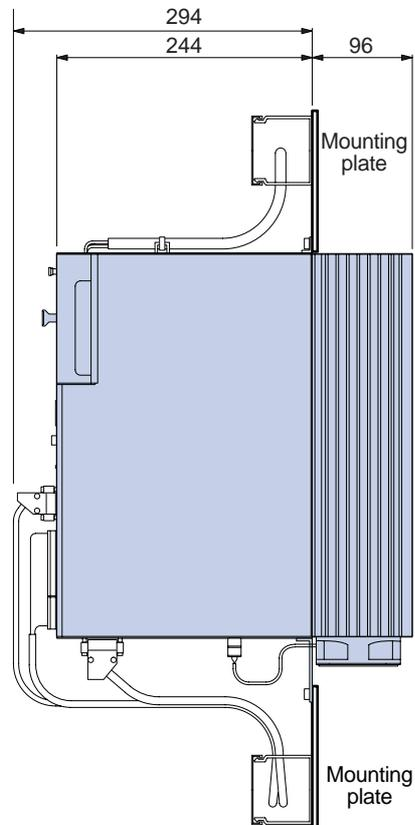
All backplate & bracket fixings accept M6 screws. For through-panel mounting, use brackets type MTS2/01
