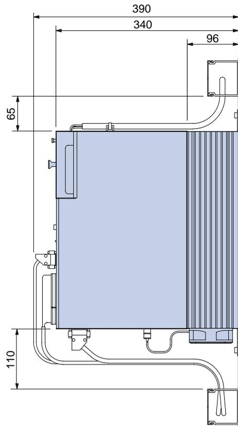
**Mounting details for through-panel mounting (not applicable to P100)**
